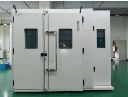
3.6 m3 constant temperature laboratory
